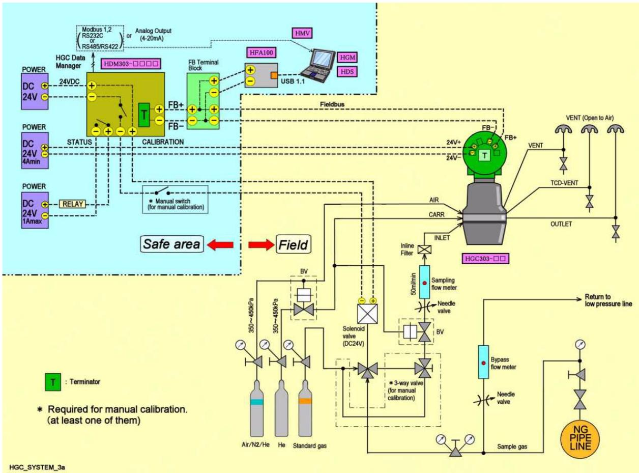
Figure 1-1 Model HGC303 measuring system diagram
