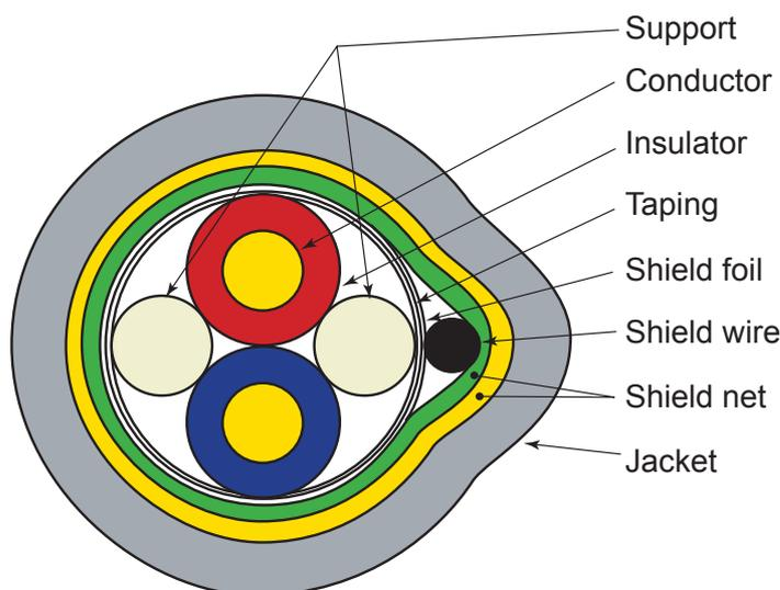
Figure 2-19 Example of Type A fieldbus cable structure
