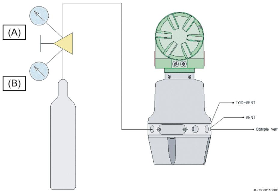
Figure 3-1 Leak check
