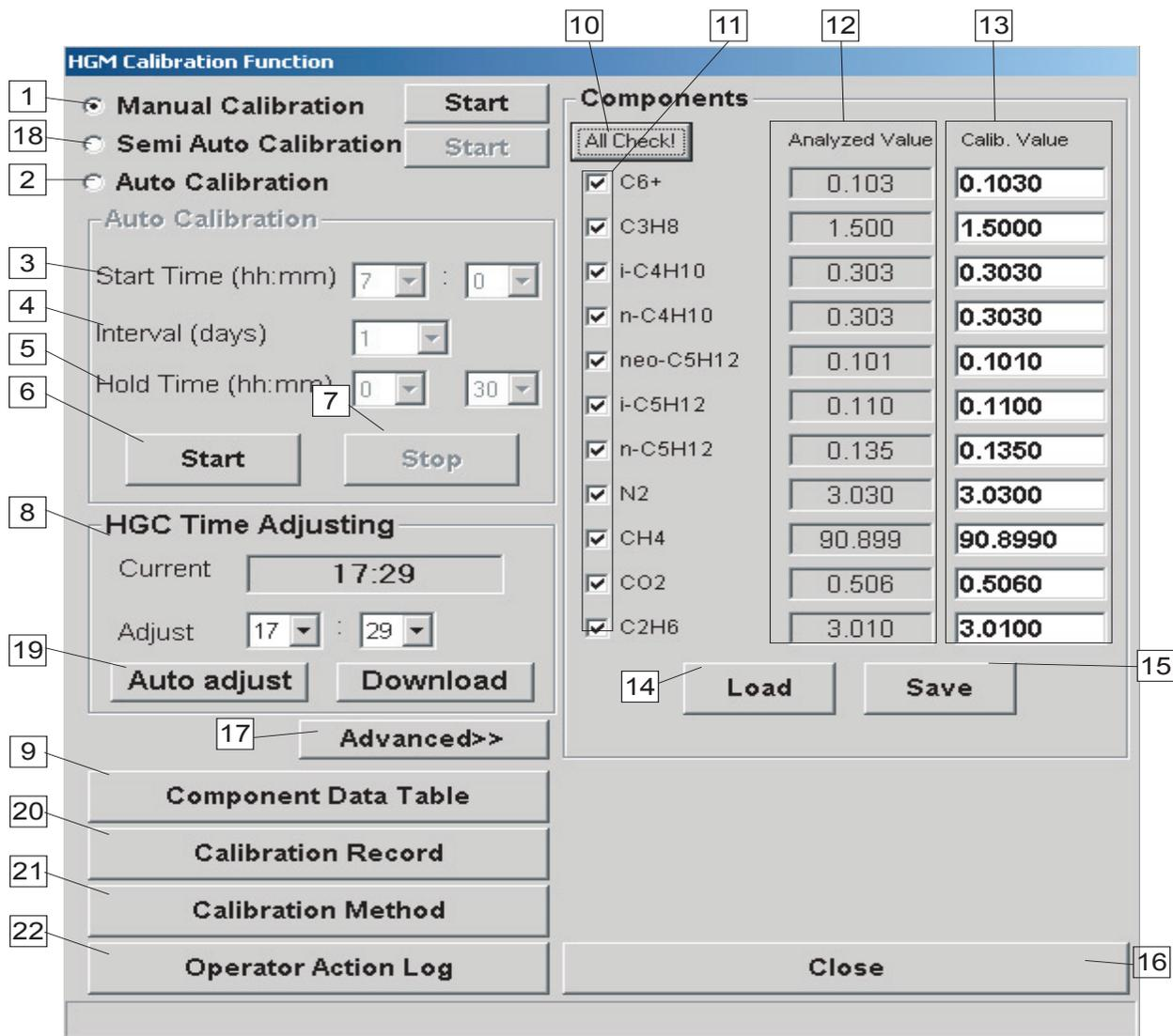
Figure 3-17 Calibration setting panel
