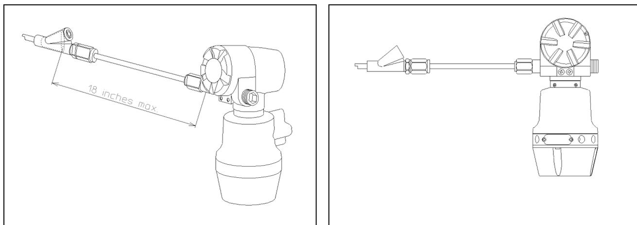
Figure S-1 An example of conduit seal (with stopping plug)
