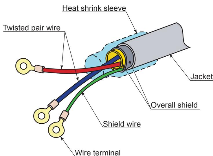
Figure 2-20 Example of cable finish
