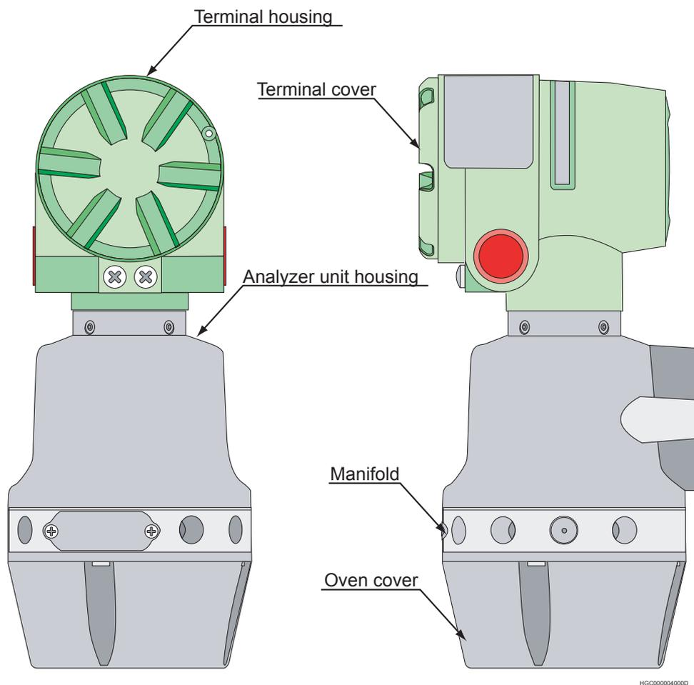
Figure 1-2 Main parts of Model HGC303
