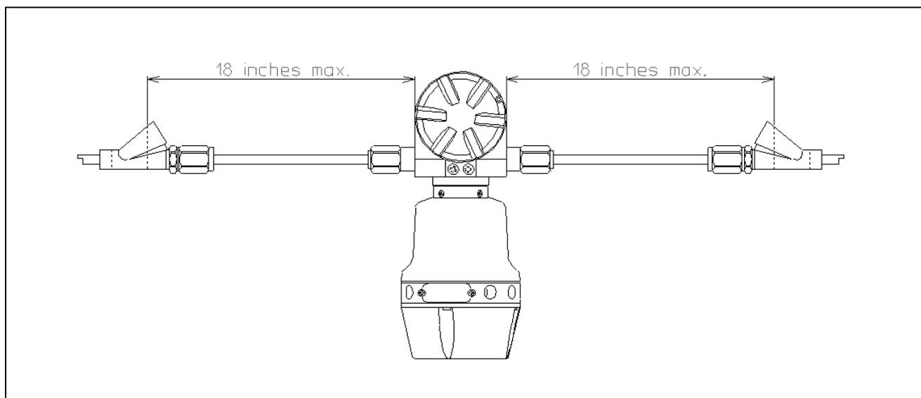
Figure S-2 An example of conduit seals (without stopping plug)
