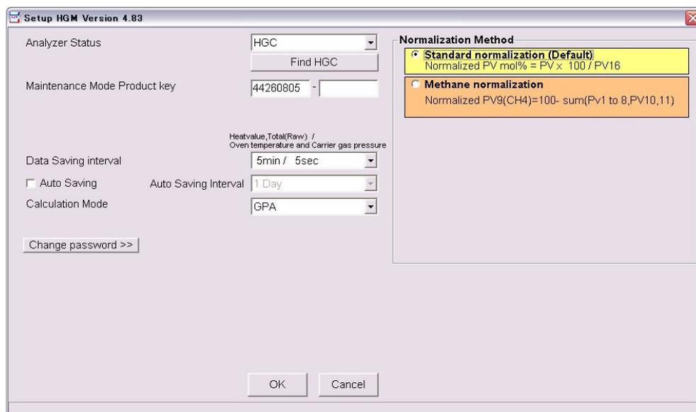
Figure 3-21 Normalization method setting (GPA)
